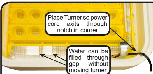
Set up incubator as shown on page 1. If you are using the automatic egg turner, place it on the wire floor in the bottom of the incubator. The thermometer should be placed directly on top of the eggs.
