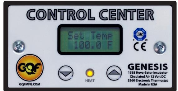
To switch the display between Farenheit and Celcius, hold both buttons down for about a second.
